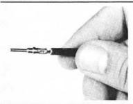
1. Grasp contact approximately (25.4 mm) one inch behind the contact crimp barrel.
