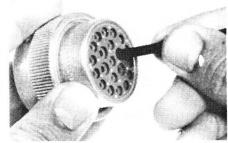
Push contact straight into connector grommet until a positive stop is felt. A slight tug will confirm that it is properly locked in place.
