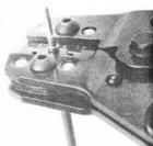
3. Close ratchet until terminal is secure and will not fall out. Place the stripped end of the wire in the crimp barrel and fully depress the tool handles. Release, and remove. If tool does not release, press further on handle.
