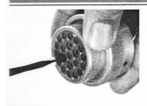
1. With rear insert toward you, snap appropriate 2. Slide tool along wire into the insert cavity size extractor tool over the wire of contact to be removed.
