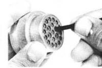
3. Push contact straight into connector grommet until a positive stop is felt. A slight tug will confirm that it is properly locked in place.
