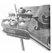
Close ratchet until terminal is secure and will not fall out. Place the stripped end of the wire in the crimp barrel and fully depress the tool handles. Release, and remove. If tool does not release, press further on handle.
