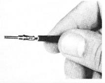
Grasp contact approximately (25.4 mm) one inch behind the contact crimp barrel.
