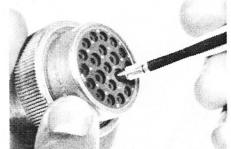
Pull contact-wire assembly out of connector.
