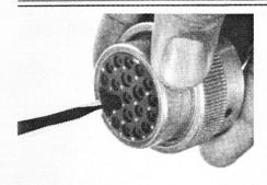
With rear insert toward you, snap appropriate size extractor tool over the wire of contact to be removed.
