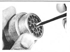
Slide tool along wire into the insert cavity until it engages contact and resistance is felt. NOTE: Do not twist or insert tool at an angle.
